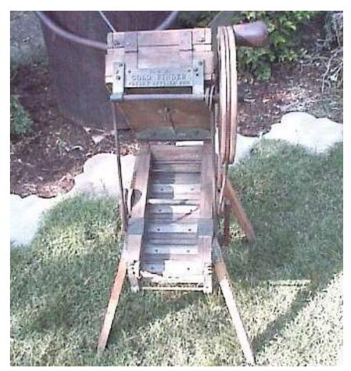
The air is created by the heavy canvas bellows at the bottom. The bellows is connected to a crankshaft (the small wheel at the bottom) which is leather belt-driven by the large hand operated wheel at the top of the drywasher. When the wheel is turned at a high rate of speed it develops a strong flow of air that literally blows everything but heavy metals clear off of the riffle box.
