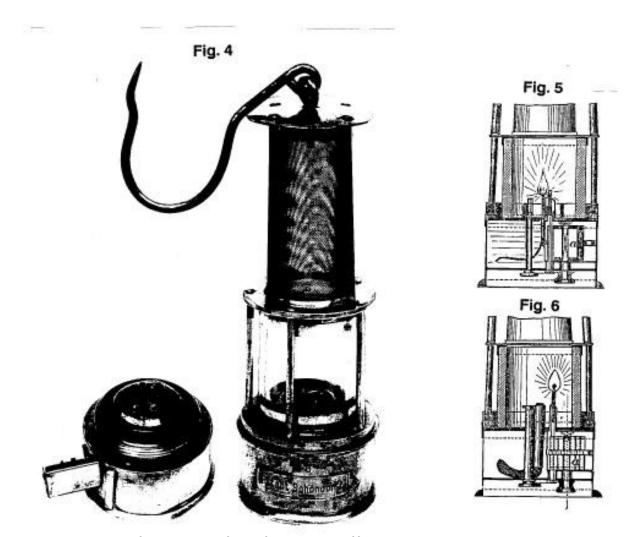
**Fig. 4** shows the oil safety-lamp of Wolf-Schondorff with magnetic lock. It was patented in 1890. The lamp can be re-ignited by using matches. The container holding the matches will be interposed lateral into the oil or fuel vessel. Each of the matches can be pushed through by a rod in right position and than can be frictioned by a toothed rod adjacent the wick.
