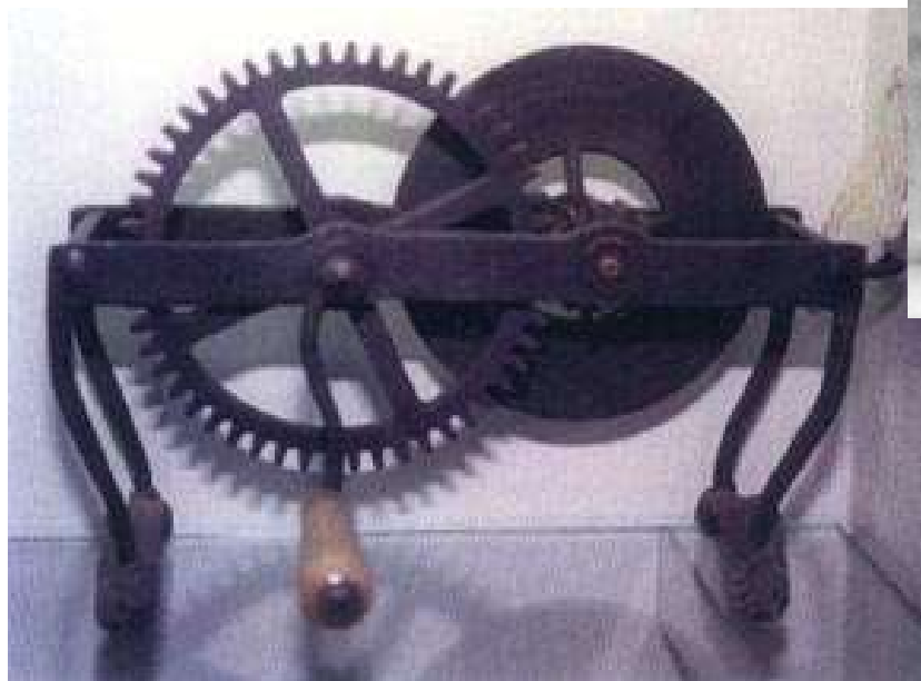
(above) Brass frame and gears, steel wheel, Beamish Open Air Museum, County Durham, England. Photo by Robert Cross.
