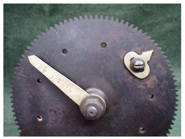
This is a close up photo showing the Level Indicator Dial. Note the hash marks scratched into the dial to let the hoist man know the exact location to stop the hoist. They are in the middle of the 100' level and just passed the 200' level.
