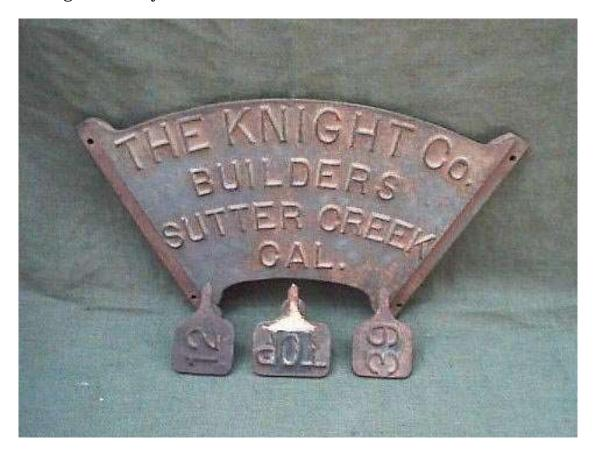
This is the original Knight Foundry cast iron name plate that was mounted on the Argonaut Hoist Indicator. It was part of the dial that the markers are mounted on. It is 23" across and 1/2" think. It weighs around 40 lb. and painted gray the same color as the hoist.
