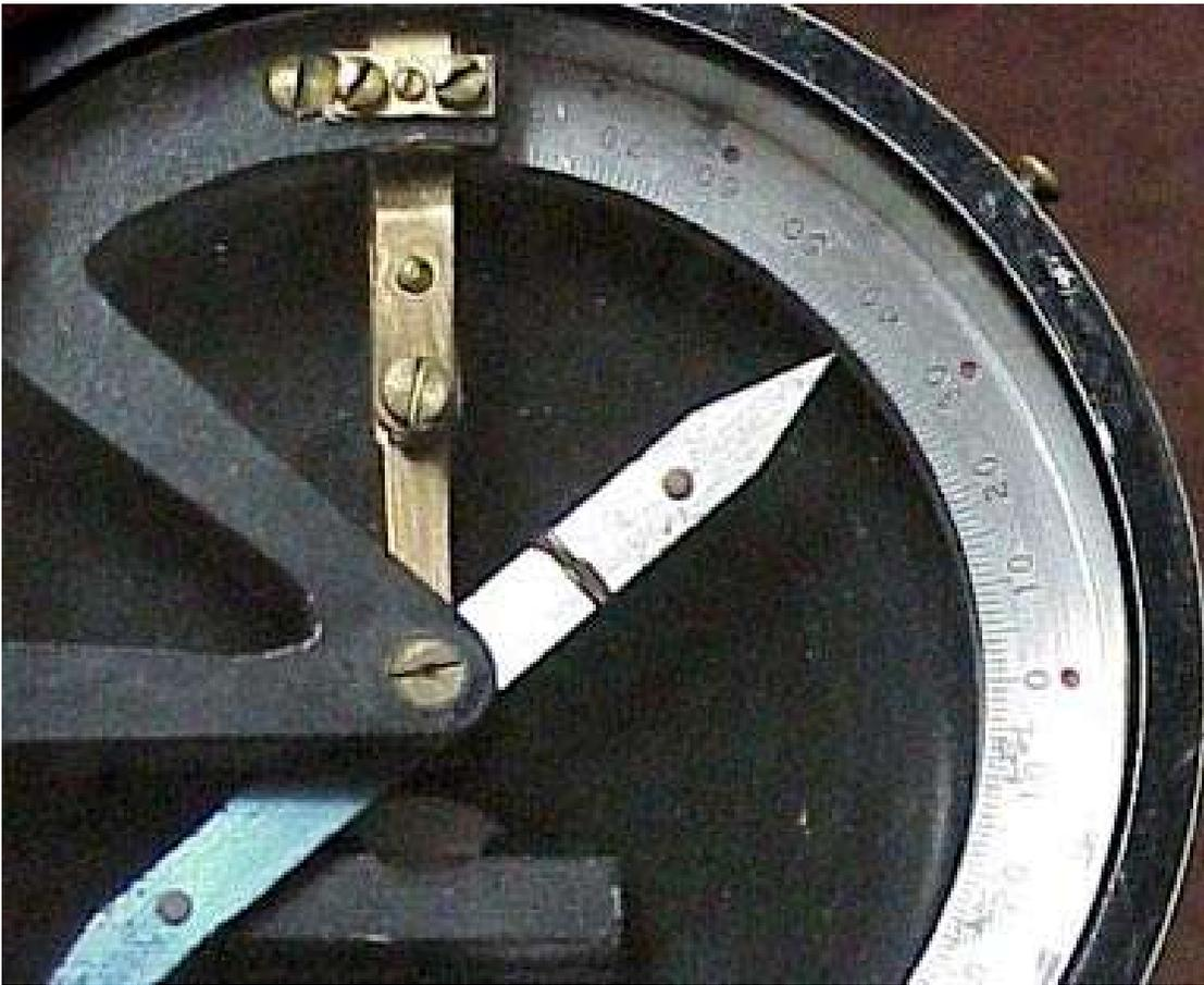
The miners' dip needle shown here, manufactured by Gurley, is unique in that it is labeled as a "Gurley Dip Needle Lake Superior Model". It is the only dip needle model I am aware of that has a regional designation. The origin of the model name is not difficult to surmise, the Michigan, Minnesota and Wisconsin
