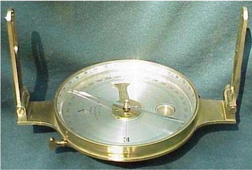
Finding mining artifacts for one's collection is always exciting but finding mining artifacts that have provenance linking them to a specific mine or mining company is doubly exciting. The two mine surveying compasses pictured and described here are two such artifacts.
