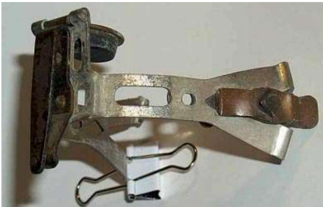
Here are some other photos showing the details of the removed brace. Seen from the inside, the top photo shows professional workmanship of the riveting, and in the lower photo, traces of black paint remain on the steel spade as on the hook equipt models.
