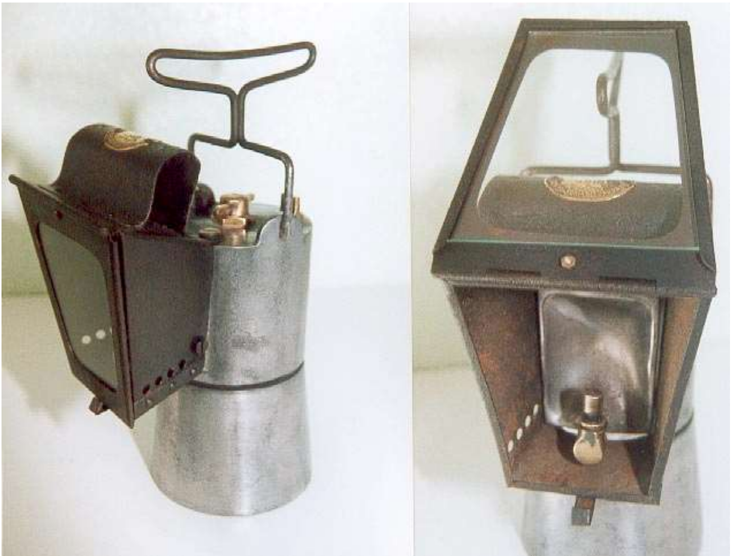
Pictures: - The 'Imperial Light lamp and the same with it's hood open showing the internal cast reflector.
