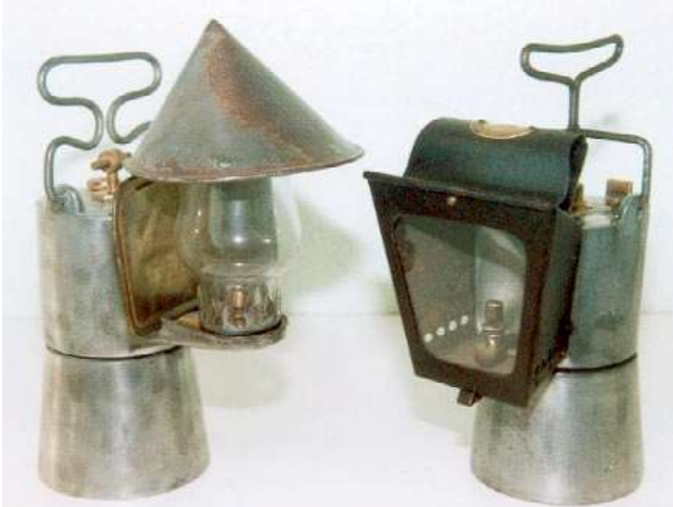
Picture: - The 'Imperial Light lamp (right), shown in comparison with the similar cast body version supplied by 'Thorn and Hoddle'
