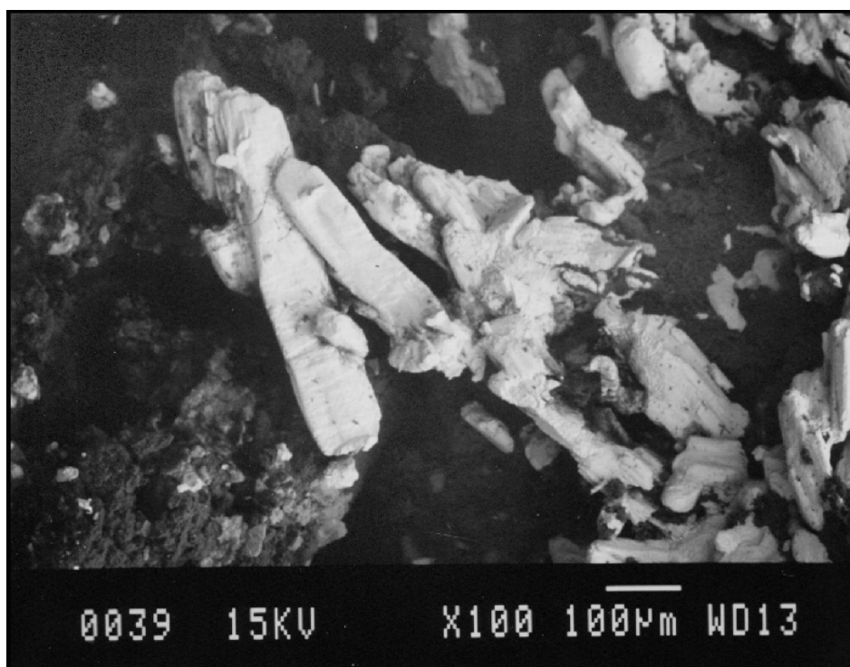
Figure 8. Isolated elongated grains of junosite exposed by etching from limestone (Silver Spoon mine). G. Dunning SEM image.
